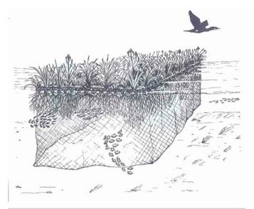
The above sketch is showing the underwater sight of a net curtain attached to a floating island to keep cormorants away from fishing under the island.
